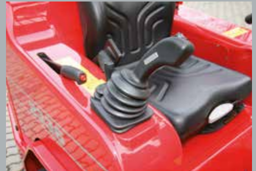
The slightly twisted joystick position simplifies operation.
